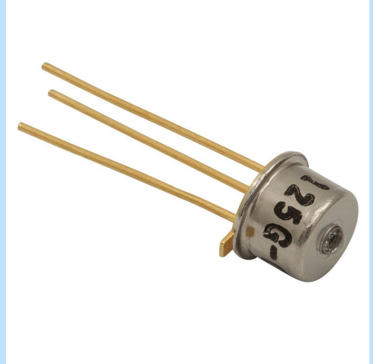
Figure #. Photodiode purchased from Thorlabs
